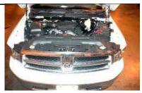
Locate the eight push pins located at the top of the grill on remove them.
