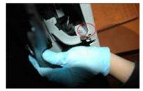
Pull back the wheel well cover to expose the single 10mm bolt and remove it.
