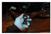
Unclip the parking bulb from wire harness.
