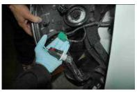
Twist off the parking bulb and disconnect the head light wire harness.
