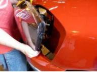
Step 15: Put the new head light into the vehicle and reverse steps to put the light back in.
