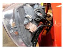
Step 5: Remove the head light from the vehicle.
