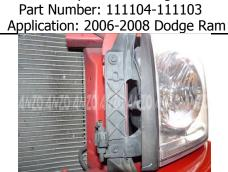
Step 1: Use the 10 mm socket to remove the two screws holding the headlight to the frame.
