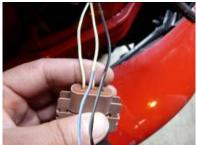
Step 11: Splice the blue wire into the middle white/green wire and the black to the black wire to power the halos.
