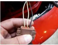
Step 10: For 2007-2008 trucks you will have to splice the halos. Pull back the cover to expose the wires on the corner parking light.
