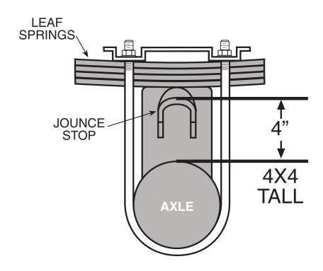
On some models with the tall jounce bumper stop, the lower bracket will have to be modified to fit level with the axle.
