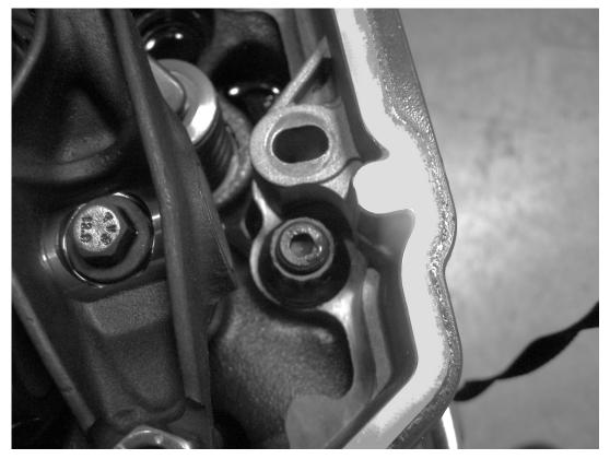
Finished machine work should allow easy removal and installation of the head stud.
