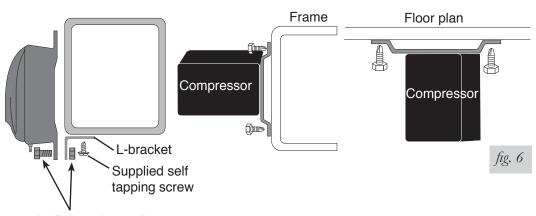
1/4" Bolt and nut will need to be provided if the L-bracket is fabricated.
