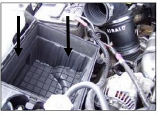
8. Install Airaid intake assembly in place of the factory air box lid & tighten factory hose clamp on intake tube to Airaid system.
