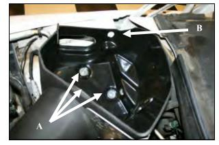
8. A) Determine the stud size of your particular vehicle, and secure the CAB using the appropriate washers and nuts. Vehicles with SAE studs will use the 1/4" x 20 Flanged Nuts (#10) and three Fender washers (#11). Vehicles with Metric studs will use the 6mm Flanged Nuts (#9) and three Flat Washers (#11). B) Re install the Factory 8mm bolt thru the CAB and into it's original location.
