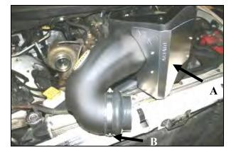
5. A) Install the aluminum Heat Shield (#4) onto the CAB using the four 1/4" Button head Bolts (#7)
