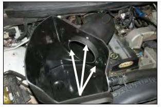
4. Attach the Intake Tube (#2) to the Cool Air Box, (CAB) (#3) using three 1/4" Button Head Bolts (#7)
