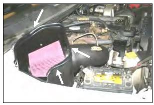
9. Install the Airaid Premium Filter (#1) onto the Intake tube as shown and tighten the clamp. Install the Weatherstrip (#6) onto the top edge of the CAB staring from the front and work your way back
