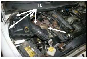
Disconnect the negative battery cables. 1. A) Loosen the hose clamp on the factory turbo inlet tube. B) Unfasten the Four clips on the right, left, and back side of the airbox. Remove the airbox lid and tube as an assembly and set aside.
