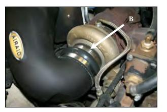
7. A) Install the CAB and Tube assembly onto the turbo inlet first, then rotate the assembly downward onto the inner fender studs. B) Secure the Silicone reducer to the turbo inlet using the # 64 Clamp (#13). C) Fully tighten the three 1/4" Button Head Bolts from step 4. Apply the Airaid Bubble Decal onto the Intake Tube as shown.
