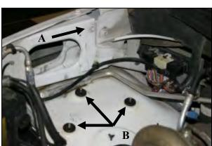
6. A) Remove the Factory 8mm fender bolt and set aside, it will be reused later in step 8. B) Place the
