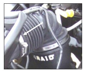
**12.** Slip the intake tube onto the air filter adapter, and tighten the clamp.
