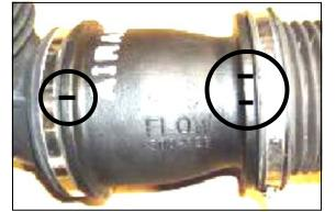
4. A.) Loosen the hose clamp that secures the facto ry airbox lid to the intake tube assembly, and remove the assembly from the lid. B.) Loosen the hose clamps above and below the factory silencer tube. Remove the factory silencer tube, and save the factory intake tubes.
