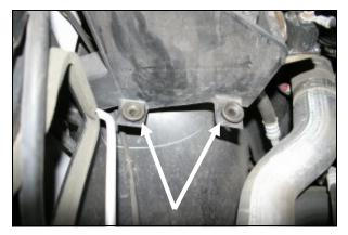
4. Remove the two grommets that held the factory
