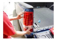
Step 9: Place the LED taillight into the truck housing, secure with screws.
