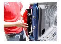
Step 3: Remove the taillight by pulling straight out.
