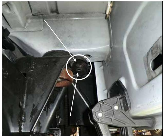
Step 1: Looking at the driver's side of the truck, at the back of the cab on the outside of the frame rail, you will see a body mount with two (2) holes on the outer lip.
