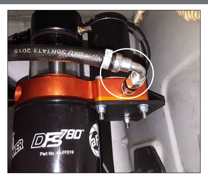
Step 18: Install the fuel inlet hose (silver 90° -6 AN fitting) onto the male -6 AN fitting on the fuel inlet port of the fuel manifold assembly and tighten.
