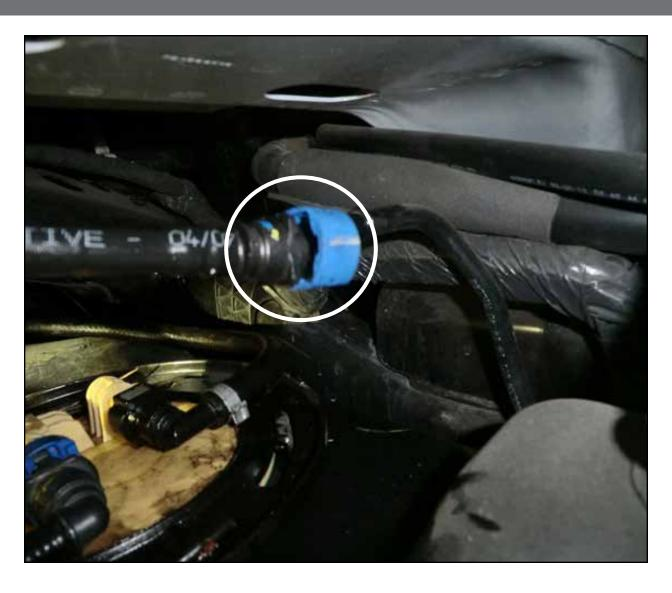
Step 11: Disconnect the factory fuel line from the fuel line near the frame (blue).
