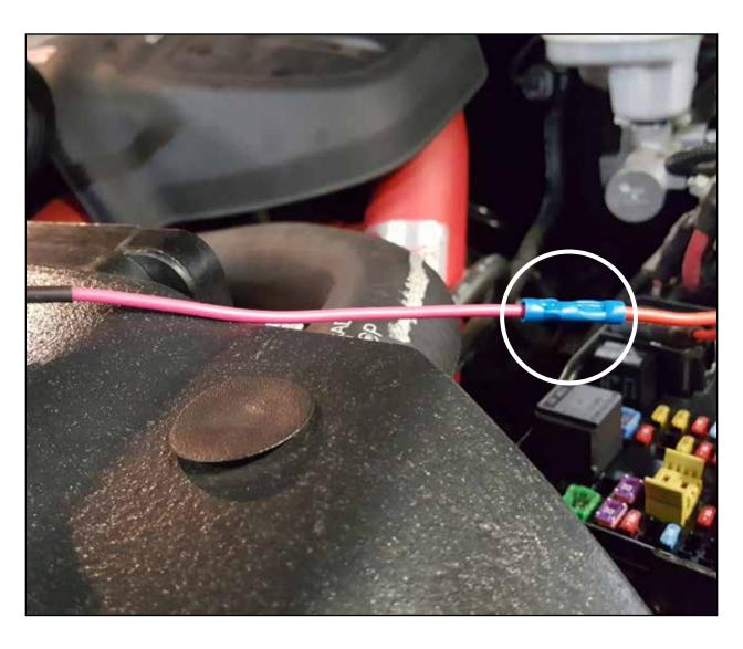
Step 35: Attach the power wire from the relay to the add a harness fuse adapter.
