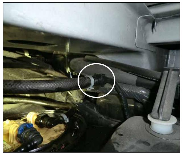
Step 14: Install the female quick disconnect fitting on the supplied fuel outlet hose (black 90° -6 AN fitting - shown below) onto the male side of the stock fuel feed line.
