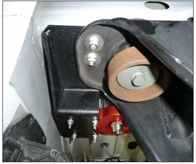
Step 4: Mount the carbon steel frame bracket and the supplied fuel manifold assembly to the frame using the supplied hardware and tighten.
