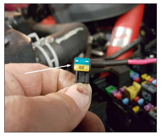
Step 36: Install the fuse removed in Step 34 and insert it into the open location on the add a harness fuse adapter (not in line with the wire).
