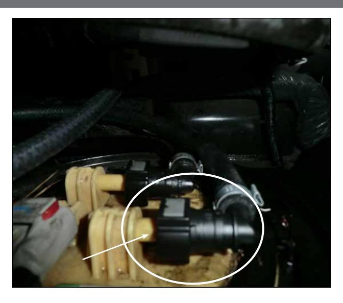
Step 16: Install the 90° female quick disconnect fitting onto the male fuel return connection on the tank.
