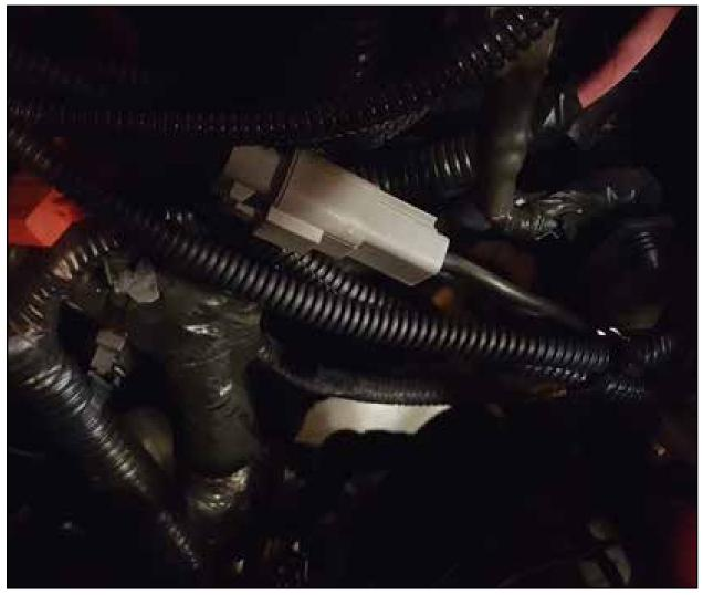
Step 31: Plug the supplied relay harness into the Deutsch connector on the power harness.
