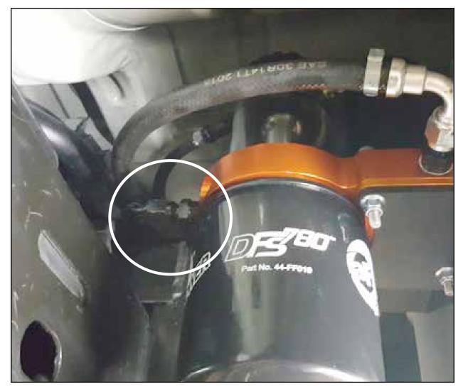
Step 19: Install the fuel outlet hose (black 90° -6 AN fitting) onto the male -6 AN fitting on the fuel outlet port of the fuel manifold assembly an tighten.
