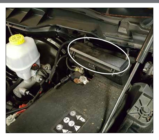
Step 28: Reinstall the power distribution box back in its factory location.
