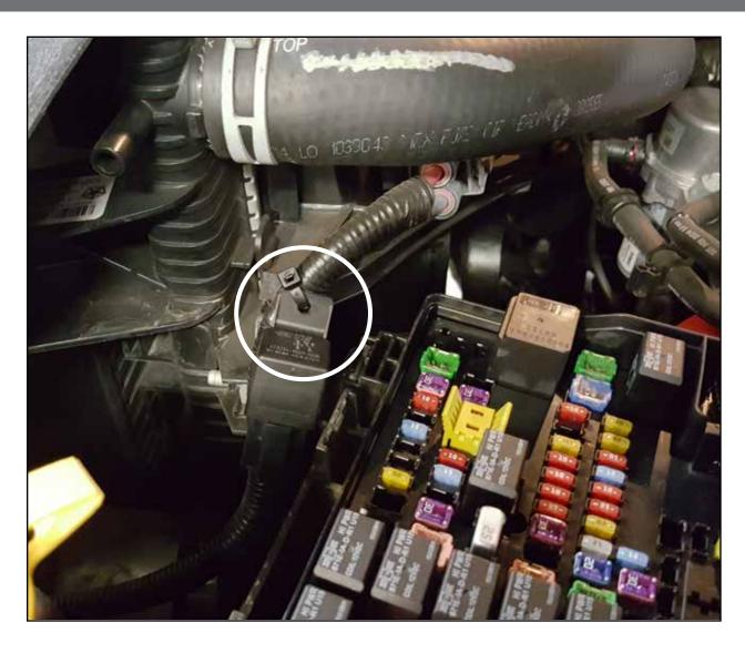
Step 32: Secure the supplied relay using a supplied nylon cable tie.
