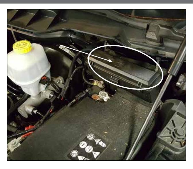
Step 26: Move the power distribution box out of the way by carefully pulling straight up on it.
