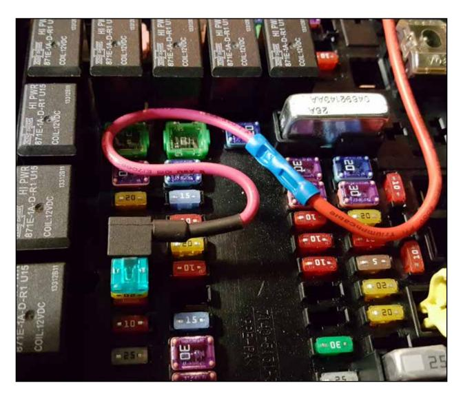
Step 37: Install the add a harness fuse adapter (with installed fuses) into the 12-volt source location chosen in Step 34.
