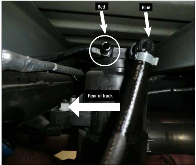
Step 12: Disconnect the factory fuel line (blue) from the factory fuel filter. Remove the line from the truck. The (red) fuel line will stay in the factory location.
