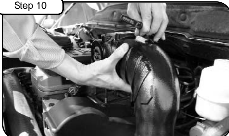
Step 10 Carefully Re-install aFe manifold into vehicle. Guide bolts into heater spacer. Finger tighten bolts.
