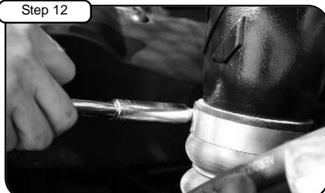
Step 12 Attach intercooler coupler back to aFe manifold. Tighten clamp w/ 11mm socket. Move back to step 11 and finish. (Do not over tighten!)
