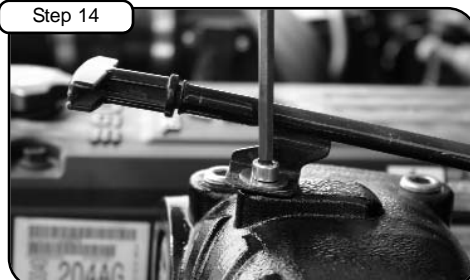
Step 14 Re-install dip stick to aFe manifold using provided M6 socket cap screw and washer provided. Tighten using 5mm allen key. Re-install harness back to aFe manifold.
