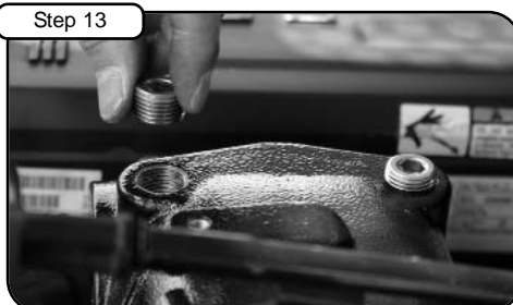
Step 13 Install the two 3/8" plugs to top of manifold. (Make sure both bolts are sealed with threadlocker). Tighten using 8mm allen key.
