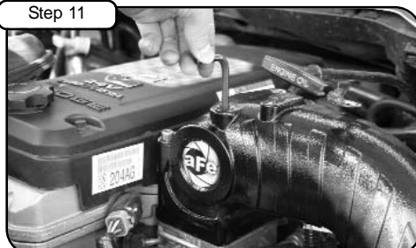
Step 11 With M8 allen key or allen key socket, tighten the 4 bolts. Do not tighten completely! (Move to step 12)
