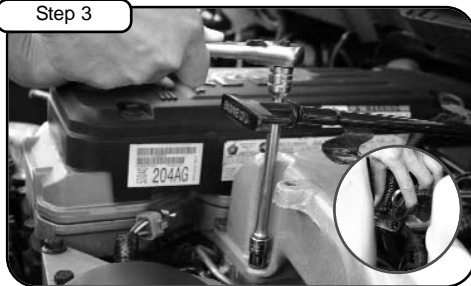
Step 3 With 10mm socket and extension, loosen the 4 bolts holding in OE manifold. (Warning: may require some force) Pull harness away in back of manifold.
