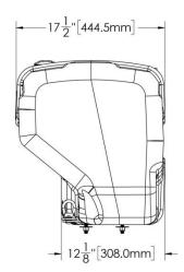
Fill Neck Throat = 1 3/8" diameter, to fit standard dispensing nozzles.
