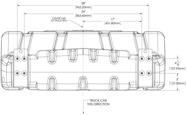
(Fig. 3) Mounting bracket bolt hole pattern for 40 Gallon, Travel Trekker, Model 5410040.
