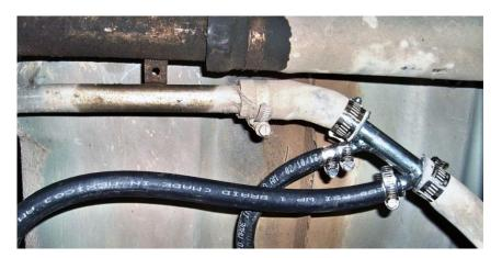
(Fig. 13) Vent Line Filler Neck Adapter (99 0000 0409) with 5/8" barrel with 3/8"and 5/16" barbs.
