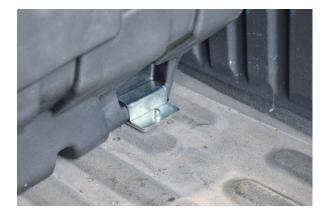
(Fig. 11) Toe clamps installed on Mounting Brackets
