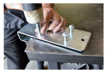
(Fig. 6) Use a deep socket to install Push Nut Retainer on 3/8"carriage bolts as shown.
