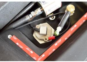
(Fig. 9) Showing grounding wire attached to the Electronic Level Sensor.
