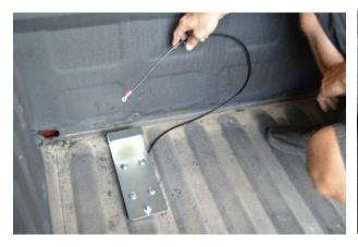
(Fig. 8) Driver's side Mounting Bracket installed. Note the ground wire attached to front inside bolt. The other end attaches to the Electronic Level Sensor on the tank.
