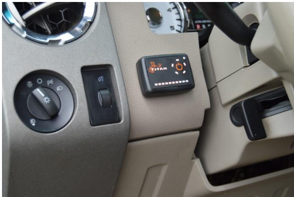
(Fig. 18) TITAN™ Electronic Controller mounted on dash.
