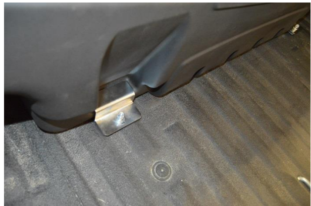
(Fig. 11) Toe clamps installed on Mounting Brackets
