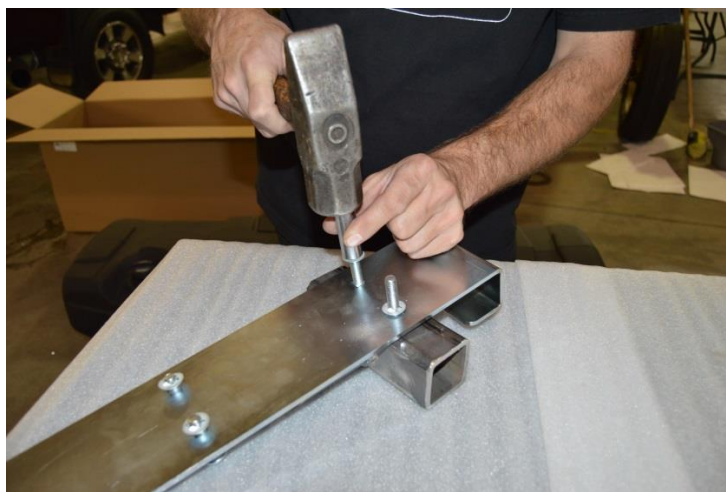
(Fig. 6) Use a deep socket to install Push Nut Retainer on 3/8\"/>
