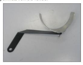
12. Install the supplied saddle clamp onto the tube mounting bracket (07160) using the provided hardware as shown.
