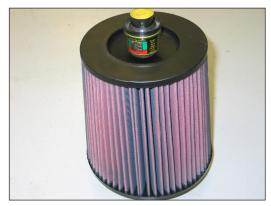
25. Install the grommet and filter minder removed in step 24 into the  $K\&N^{\textcircled{R}}$  air filter as shown. On vehicles not equipped with filter minder install the provided plug.
