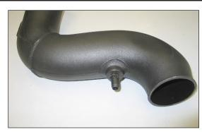
26. Install the provided ¼"npt fitting into the intake tube as shown.
