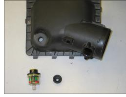
24. On vehicles equipped with filter minder, remove filter minder and grommet from the upper air box as shown.
