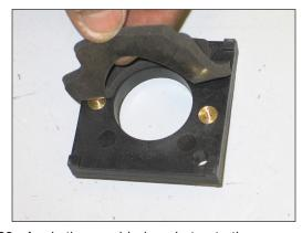
29. Apply the provided gasket onto the mass air sensor adapter as shown.
