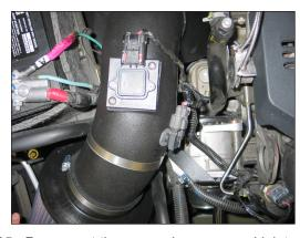
35. Reconnect the mass air sensor and inlet air temperature sensor electrical connections.
