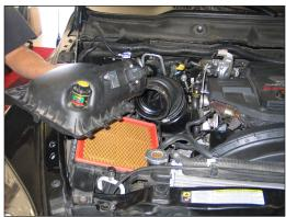
6. Remove the upper air box housing from the lower air box housing.
