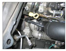
34. Install the provided air injection hose onto the air injection tube and then connect the open end to the 1/4"npt fitting in the K&N  $^{\circledR}$  intake tube.
