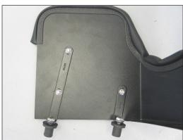
20. Attach the two provided inserted nuts to the heat shield using the provided hardware as shown. NOTE: Do note tighten the mounting bolts at this time.
