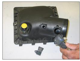
22. Remove the screws which secure the mass air sensor and inlet air temperature sensor and then remove the sensors as shown.
