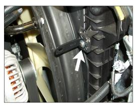
15. Remove the radiator fan shroud bolt. Then install the heat shield mounting bracket (07158) onto the fan shroud using the provided hardware as shown.
