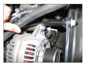
13. Remove the upper alternator mounting bolt shown.
