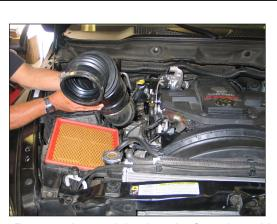
8. Remove the stock intake tube from the vehicle.
