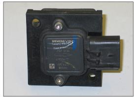
30. Install the mass air sensor into the adapter and secure with the provided hardware.
