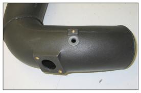
27. Install the provided grommet into the intake tube as shown.
