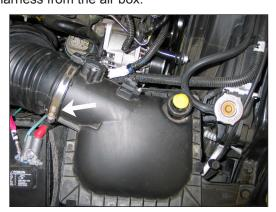
4. Loosen the hose clamp which secures the stock intake tube to the upper air box housing.
