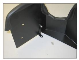
18. Install the heat shield mounting bracket (06723) onto the heat shield using the provided hardware. NOTE: The bolt should be inserted from the back side through the heat shield and then through the bracket.
