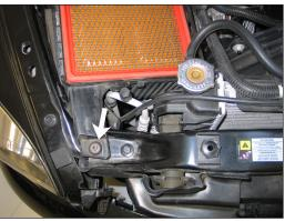
9. Remove the nut which secures the front of the lower air box housing to the radiator core support.
