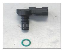
23. Remove the "O" ring from the air temperature sensor.
