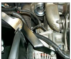
14. Install the tube mounting bracket assembly onto the alternator and secure with the factory bolt removed in the previous step.
