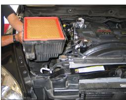
10. Firmly pull the lower air box assembly up to disengage it from the mounting grommets and then remove it from the vehicle.
