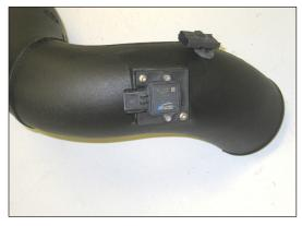
31. Install the mass air sensor assembly into the intake tube and secure with the provided hardware. NOTE: The arrow on the top of the mass air sensor should be pointed in the direction of the intake air flow, towards the turbo inlet.
