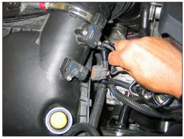
3. Disconnect the inlet air temperature sensor electrical connection and then unhook the wiring harness from the air box.
