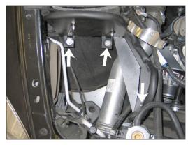
21. Install the heat shield assembly into the engine compartment as shown. The inserted nuts should be positioned into the air box mounting grommet holes and align the front mounting hole in the heat shield with bracket installed in step #15. Secure the heat shield with the provided hardware and the two inserted nuts.
