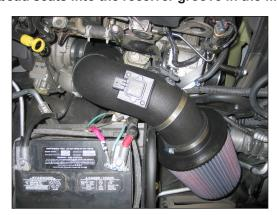
33. Install the intake tube and filter assembly, slide the intake tube into the silicone hose at the turbo and then align with the saddle bracket. Secure the assembly with the provided hose clamps.
