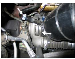
7. Release the tension on the air injection vent hose clamp and the hose clamp which secures the intake tube to the turbo inlet.
