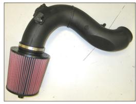
32. Install the K&N<sup>®</sup> Air Filter onto the intake tube and secure with the provided hose clamp.
