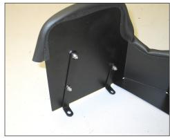
19. Install the provided heat shield mounting bracket (06722) onto the heat shield using the provided hardware.
