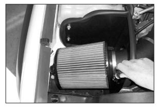
25. Install the K&N<sup>®</sup> air filter onto intake tube as shown then tighten completely.
