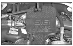
4. On 2002 models, remove the torx bolt from intake resonator as shown.
