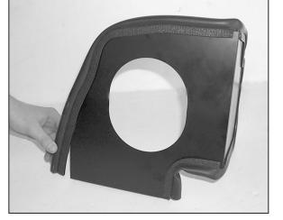
8. Apply the provided trim seal to the heat shield assembly as show. Trim if necessary.
