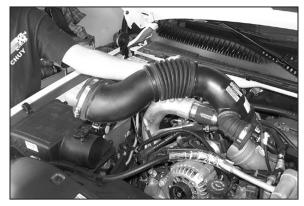
6. Loosen hose clamp at intake manifold and airbox, then remove complete air intake tube.
