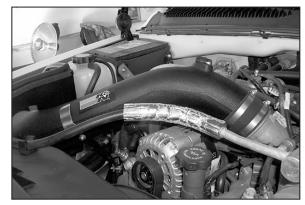
20. Secure the K&N<sup>®</sup> intake tube to the intake manifold with the provided hose clamp.
