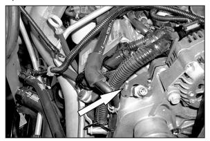
12. Remove nut from the Schrader valve as shown.
