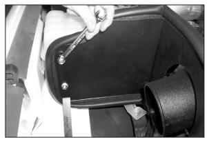
22. Adjust heat shield and bracket for necessary clearance, then tighten all hardware completely.
