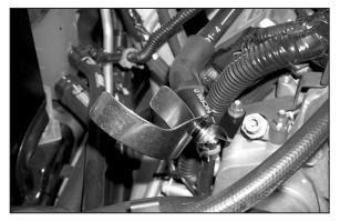
14. Secure bracket onto stud and secure bracket with nut that was removed in step 12. Do not tighten completely.
