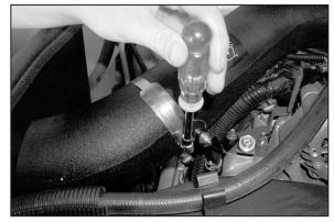
21. Install saddle bracket onto intake tube with hose clamp provided. Adjust for best fit and tighten all hardware.
