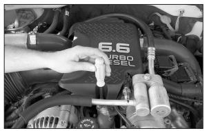
3. On 2001 models, remove the 8mm bolt that retains the engine cover, then remove cover.
