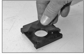
17a. Install the provided gasket onto the K&N<sup>®</sup> mass air sensor adaptoras shown.
