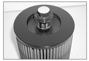
24. Install filter restriction gauge onto air filter as shown.
