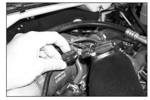
26. Reconnect the mass air sensor electrical connection as shown.
