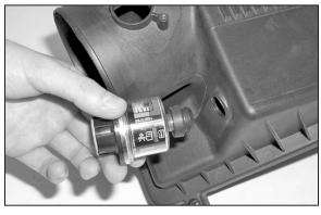
16. Remove the restriction gauge and grommet from the stock airbox assembly as shown.
