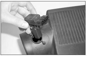
15. Loosen and remove the two torx screws that retain the mass air sensor with the provided torx wrench, then remove sensor.
