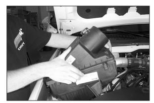
7. Pull firmly upwards on stock airbox to remove from vehicle. **NOTE: K&N Engineering, Inc., recommends that customers do not discard factory air intake.**
