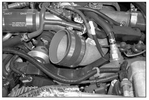
19. Install silicone hose onto intake manifold with provided hose clamps.
