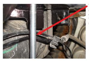
The carriage bolt is always on the outside of the brake line on the passenger's side, regardless of the year.
