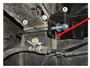
Draw hardware evenly (snug only, do not tighten yet) making sure the lower bracket stays in position and locked around the U-bolts.
