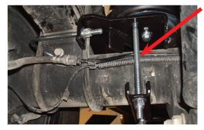
Check driver's and passenger's sides to make sure the hard brake line is not rubbing on the carriage bolts. Adjust by pushing on the line to gain clearance if necessary.
