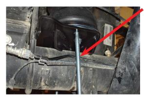
Carriage bolt must be on the outside of the hard brake line and axle for this model that has the brake line flush to the axle.
