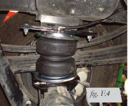
Inside view of the passenger's side installation.
