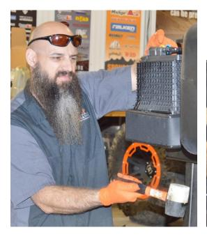
(Fig 8) Using a rubber mallet, <u>carefully</u> tap the water separator up and out of its mounting bracket on the OEM tank.
