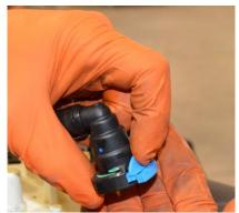
(Fig. 7): **Method for Disconnecting Fuel Line Couplings:** The majority of the couplings involved in this installation are of the quick connect type shown in left photo above. To disconnect, a) Slide the tab that has teeth on its edge outwards as shown in the center photo. b) Next, press the rounded button, as shown in the right photo, and pull the coupling apart. The coupling shown in Fig. 5 functions differently, see Step no. 9 for it.
