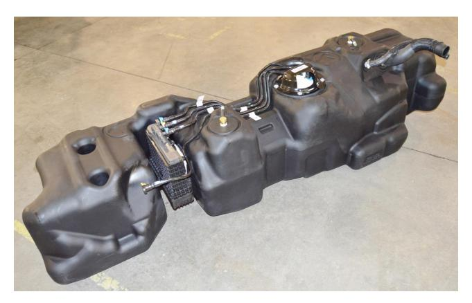
(Fig. 13) TITAN 7020217 tank shown with sending unit, water separator, fuel lines, sending unit guard, and fill and vent hoses installed; ready for installation into the vehicle.
