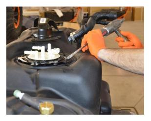
(Fig. 12) Reuse the OEM hold-down ring to mount the sending unit in the TITAN tank. Tighten by turning it clockwise as far as it will go.
