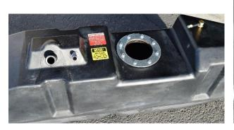
(Fig. 10) Install the OEM 1  $\frac{1}{2}$ " fuel tank fill hose to the large king nipple and the  $\frac{3}{4}$ " OEM vent hose to the smaller nipple. Be sure to fasten tightly with the OEM hose clamps.
