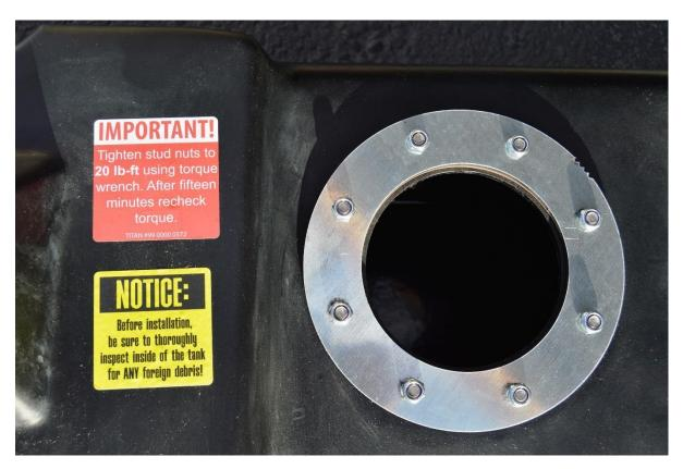
(Fig. 7) The sending unit top flange and installation notices are shown here.
