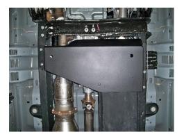
**Note:** Most late model Heavy Duty Ford truck models already have the frame drilled to accept the skid plate. If you come across a vehicle which does not, follow the placement instructions, clamp the skid plate into position and drill the bottom flanges of the frame to accept it. If your vehicle already has a factory skid plate, simply remove it and replace it with this one.
