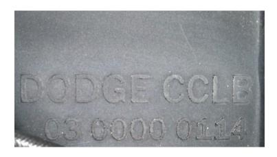
Note: The tank body has the above identification on its top. Please check to be sure the tank is properly identified as the one to fit your vehicle.
