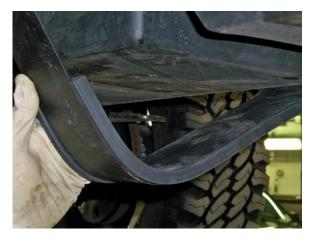
(Fig. 4) Install rubber bushings (pn 99 0000 0103) on both straps with the channel side toward the strap.
