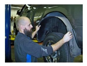
(Fig. 1) Some vehicles may require the removal of the fender liner and perhaps the left rear wheel so as to facilitate access to the tank fill and vent hoses.
