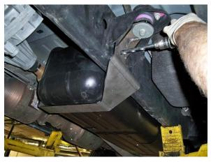
(Fig. 5) On 7030210 (Crew Cab, Short Bed) tanks only, bolt the Front Support to the nearest cab mount (as shown above), then use a  $\frac{1}{2}$ " drill bit to drill through the support hole and through the vehicle's frame. Bolt the support to the frame using the bolt and hardware provided.
