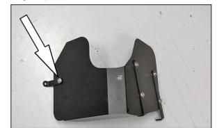
9. Install the front heat shield mounting bracket (07158) onto the heat shield using the provided hardware.
