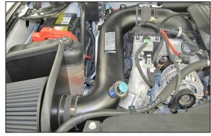
17. Install the K&N® intake tube into the hump hose at the turbo inlet and then into the hose at the filter adapter. Align the tube for best fit and then secure with the provided hose clamps.
