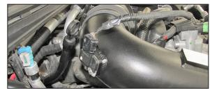
18. Connect the mass air sensor electrical connection.
