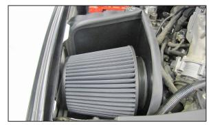
12. Install the K&N® air filter onto the filter adapter and secure with the provided hose clamp.
