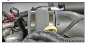
15. Install the provided hump hose (08633) onto the turbo inlet and secure with the provided hose clamp.
