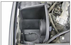
11. Install the heat shield assembly onto the filter mounting plate and secure with factory bolts from step #5.
