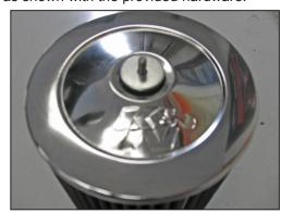
24. Install the supplied rubber washer and fender washer onto the stud protruding from the filter lid as shown.
