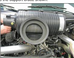
6. Remove the filter housing from the vehicle.
