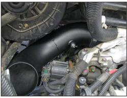
13. Install the primary K&N® intake tube (27434) into the silicone hose at the throttle body and align with the mounting bracket installed in step #12. Secure the primary intake tube with the hose clamp and hardware provided.
