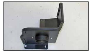
9. Install the provided filter adapter onto the heat shield and secure with the provided hardware.
