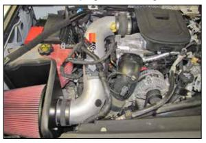
17. Install the K&N<sup>®</sup> intake tube into the hump hose at the turbo inlet and then into the hose at the filter adapter, adjust the tube for best fit and then secure with the provided hose clamp.
