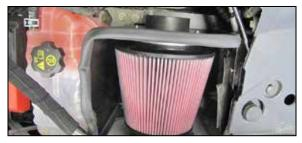
11. Flex the heat shield back and then install the K&N<sup>®</sup> air filter onto the filter adapter and secure with the provided hose clamp. Secure the heat shield with two of the factory bolts removed in step #7.
