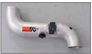
15. Install the Mass air sensor and Humidity sensor into the K&N<sup>®</sup> intake tube and secure with the provided hardware.
