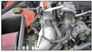
18. Reconnect the Mass air sensor and humidity sensor electrical connections.
