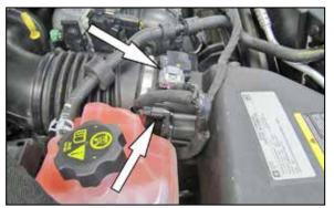
2. Disconnect the mass air sensor and humidity sensor electrical connections.
