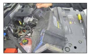
6. Lift up and remove the air box from the vehicle. NOTE: K&N Engineering, Inc., recommends that customers do not discard factory air intake.
