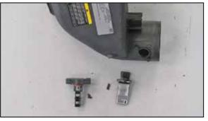
14. Remove the screws securing the mass air sensor and Humidity sensors into the factory air box and then remove the sensors from the air box.
