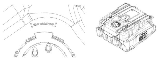
(Fig. 3) Line sending unit tab up with "TAB LOCATION" marks on tank.
