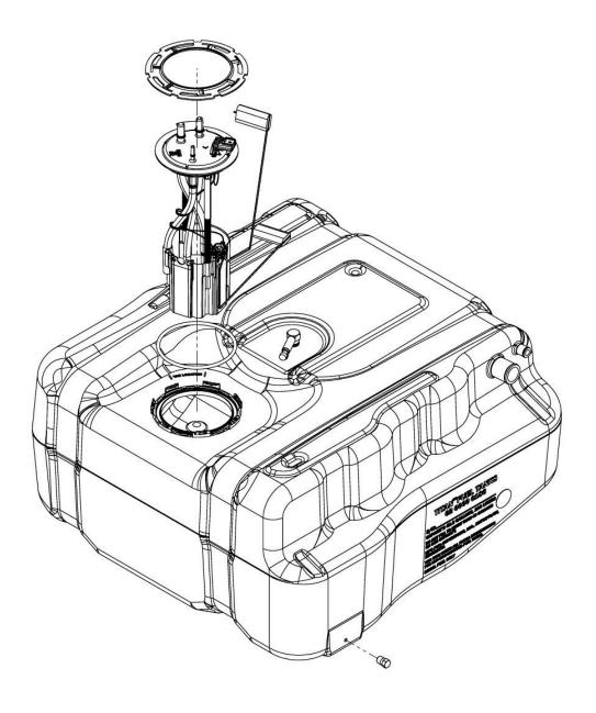
(Fig. 2) Exploded view of sending unit and proper part installation in TITAN 8020011 after-axle replacement tank.
