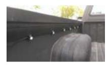
We chose to install them as bedrail lights but these Auxiliary lights can be installed any where on the vehicle.
