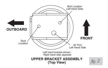
4. Set roll plate on bottom of bellows. Attach lower bracket to bottom of bellows on both units using the holes as shown (Fig. 1). The extended tabs should face rearward. Use the 3/8" lockwashers and 3/8"-24x7/8" HHCS torque to 15-20 lb.-ft. Be sure that lower bracket and upper bracket are parallel to each other as shown in Figure 2.
