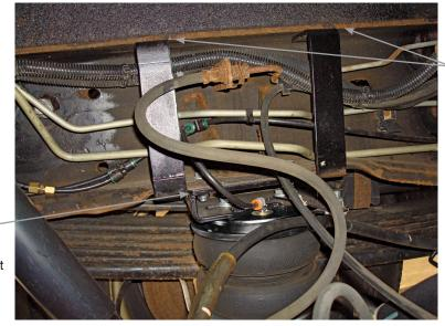
Brace on upper bracket fits under the top of the frame flange
