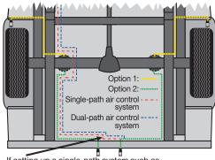
If setting up a single-path system such as Wireless One or SmartAir II, use a T-fitting to connect the two sides. Dual-path systems such as Wireless Air have separate air lines to the air control system.
