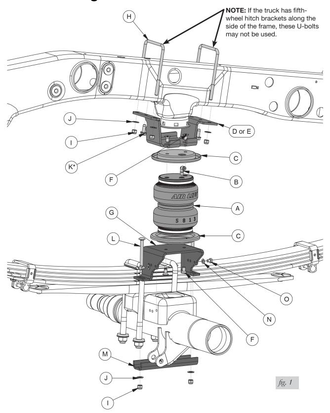
\* Optional hardware for vehicles equipped with fifth-wheel hitches that have frame side plates (see page 8 for details)
