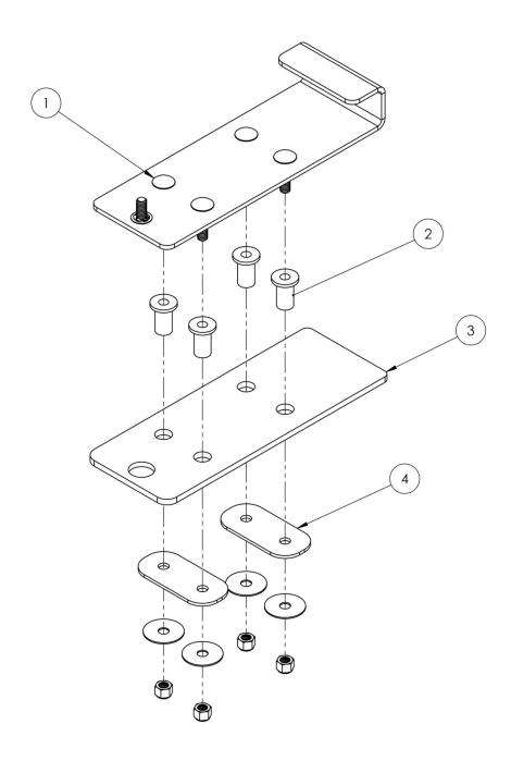
Exploded view showing proper installation of Aluminum Body Insulator Ki
