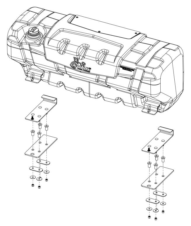
This is an exploded view showing proper installation of the Aluminum Body Insulator Kit under the tank mounting brackets on top of; and Polymer Double Washers underneath the truck bed. Be sure to see *Travel Trekker 40™* Installation Instructions.
