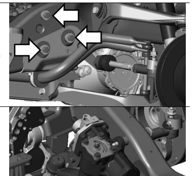
Remove the Pitman arm by removing the nut and washer (arrow shown) and using a puller tool to remove from steering gear.
