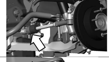
Slip outer tie rod stud into steering knuckle from below, and torque nut to specification.
