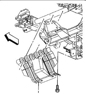
Disconnect steering damper from the Center Link.
