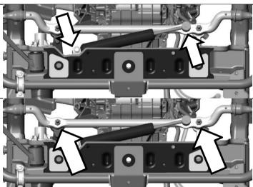
Remove center link from Pitman arm and Idler stud.
