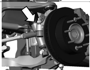
Ensure the tie rods remain near the length set earlier, and tighten the adjustment jam nut.
