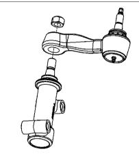
Reinstall the Idler arm assembly into the frame and torque to spec.
