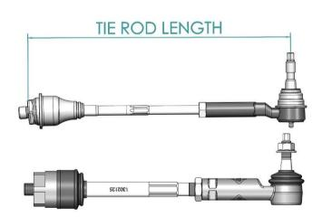
Install the inner tie rod onto the BD Center Link by threading into the link and tightening to spec.
