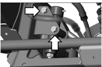
Install BD Center link onto Pitman and Idler arm studs, torque nuts to specification.
