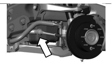
Remove sway bar end link by removing upper nut (arrow shown). Slide out bolt from below lower control arm.
