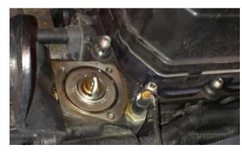
STEP 7: Remove the stock thermostat. Inspect it for wear and proper function. With a Scotch-Brite ™ pad and degreasing solution, thoroughly clean the sealing surface of the stock thermostat and thermostat housing. Be sure to remove any foreign debris, and reinstall the OE thermostat.
