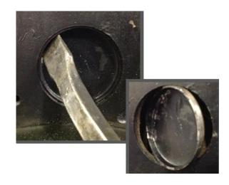
STEP 11: With the freeze plug removed, using a Scotch-Brite <sup>™</sup> pad and a degreasing solution, thoroughly clean the block surface area from the head down to the rear cover, as well as the bore where the freeze plug was previously installed. Be sure to remove any dirt or foreign debris.
