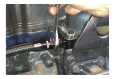
STEP 16: Utilizing the coolant bypass line riser brackets (item 11) and M8 socket head cap screws (item 5) in your kit; position the clamps over the bypass coolant line and fasten them to the cylinder head in the available tapped holes between cylinder numbers 2 & 3 as well as between cylinder numbers 4 & 5.
