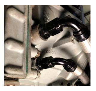
**STEP 3:** Install the transmission lines according to the figure on page 3 and routings shown on pages 5 & 6. Use the double hose clamp ties (item 6) and zip ties (item 7) to retain the hoses and prevent contact with rotating or high-temperature components.
