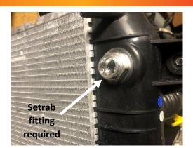
**STEP 2:** Install each of the fittings in the transmission and front mounted auxiliary cooler. Image shown at right is of an LB7/LLY vehicle.
