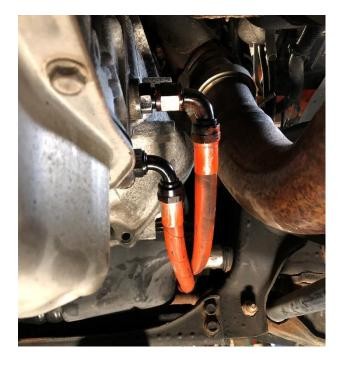
Route the lines uniformly along the passenger side of the chassis, just inside the frame rails by approximately 6-12".
