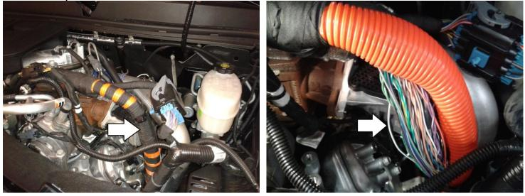
**2017-2018 GM L5P** – Locate the 8 pin sub-harness disconnect on the top of the engine for the crankshaft position sensor. Locate the solid green wire in pin 3. Remove some harness tape to have some wire to work with. Attach the light blue wire here for RPM pickup. Solder the wire and cover with heat shrink for longevity. Rewrap with tape when complete.
