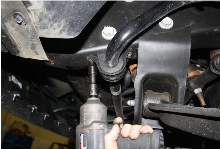
Figure 3: unbolt sway bar from frame
