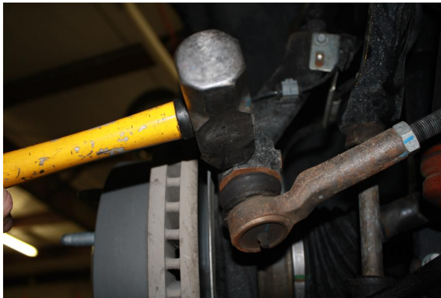
Figure 9: remove passenger tie rod from spindle
