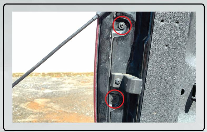
2. Insert a plastic trim tool in the gap shown below and pry the tai light backwards away from the bed.
