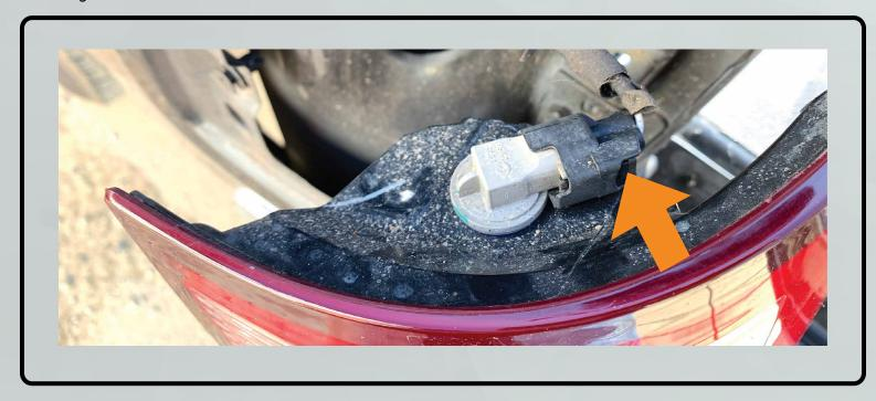
5. Grab one Morimoto tail light of the same side, locate the included incandecent adapter and plug it into the Morimoto tail light (#1). The other side of the adapter plugs into the OEM harness (#2).
