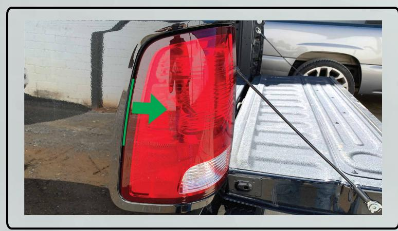
3. Unplug the brake light connector by first releasing the locking tab (#1). Then press on the tab (#2) to release the clip and slide the connector off.
