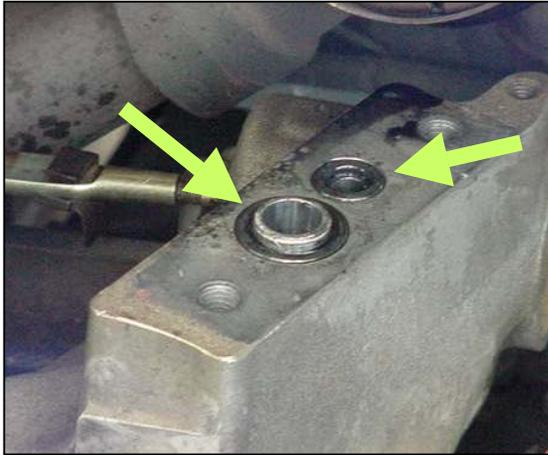
12. Ensure the 2 supplied o-ring oil seals are properly seated on the pedestal.. The turbo oil drain hole will pilot on the raised sleeve.
