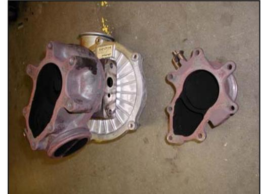
11. Remove the backpressure valve assy from the old turbo and install on the new turbo. Use anti-seize compound on the threads & torque the bolts to 185 - 215 lb-in.
