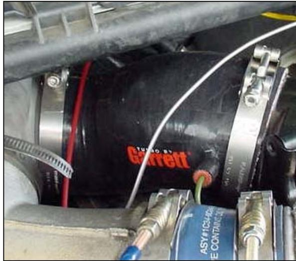
21. Double check that the compressor inlet area is free from any foreign objects and that the inlet hose is clean. Install the new compressor inlet hose in place and insert the green hose into the boss. Tighten clamps snugly.
