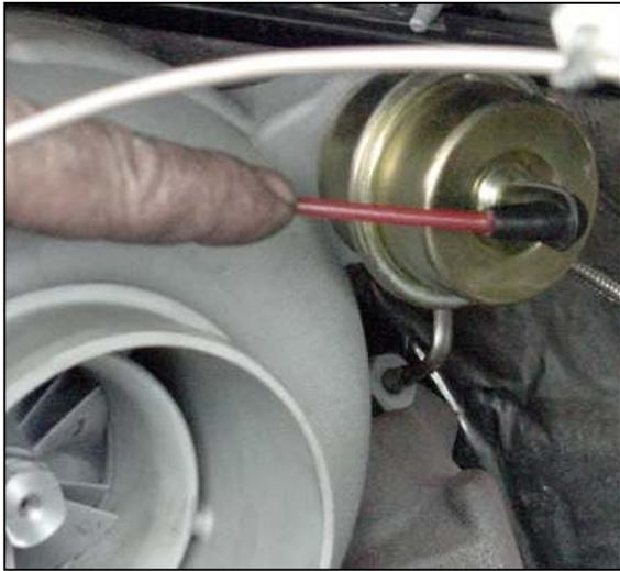
20. Re-install the red wastegate hose onto the wastegate hose actuator
