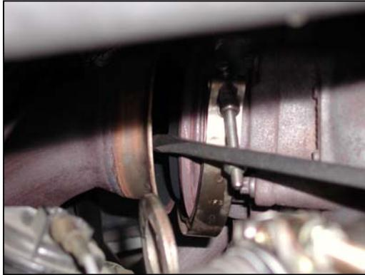
6. Using a 7/16" deep socket, loosen turbine outlet v-band clamp and move clamp off of the flange. Separate down-pipe from turbo
