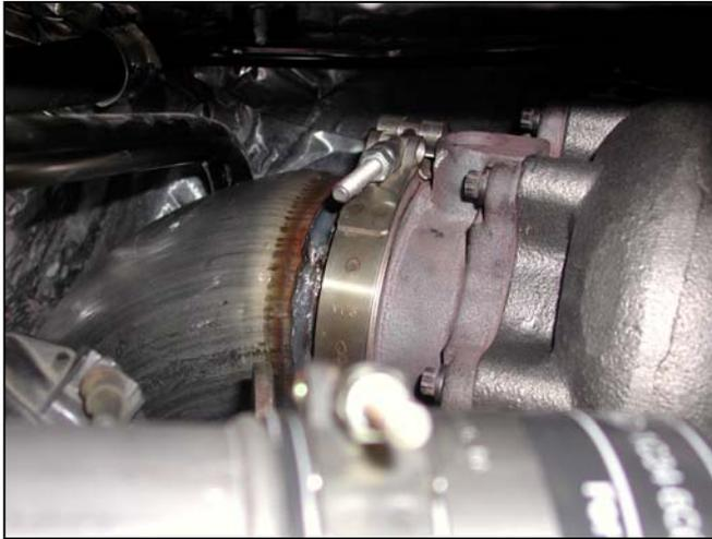
17. Install downpipe. Guide the v-band flange to mate with the turbine discharge flange. Install v-band clamp & torque to 110-130 lb-in.
