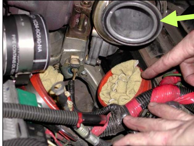
18. Remove covers (rags in this picture) from the intake manifold openings. Re-use the original compressor discharge O-ring and mount it into the new compressor discharge groove. A light coating of RTV or grease can be used to hold it in place.
