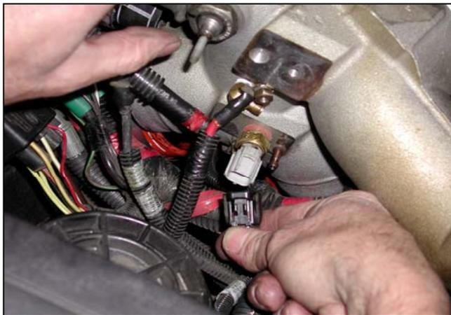
19. Position the x-section pipe in place and re-install hoses. Tighten compressor discharge v-band clamp to 110-130 lb-in. Tighten hose clamps to 50-60 lb-in, and re-install all electrical and temperature connections.
