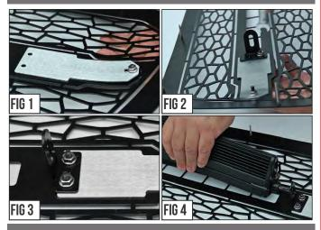
Put into place one of the Bracket Tabs and seucre with provided Hardware as seen in Fig. # 2-4 and then from the backside of grille position LED Light Bar.
