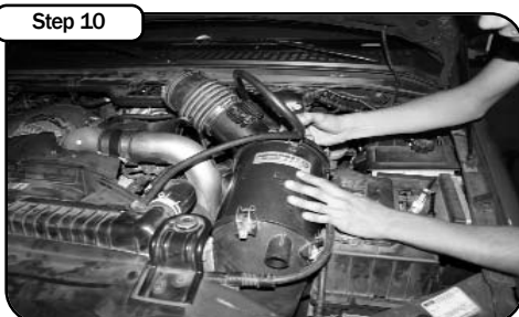
Step 10 Carefully install the air box outlet. Make sure the tangs engage on the bottom of the air box. Check to make sure the clamps are tight.
