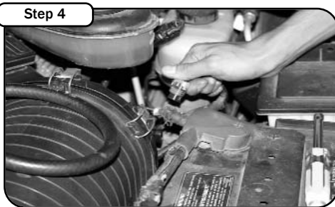
Step 4 Disconnect the Filter Minder located on the back of the air filter box.
