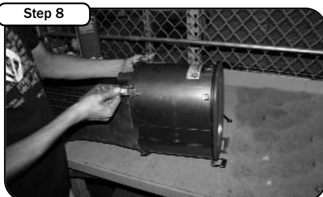
Step 8 Transfer the inlet portion of the air box to the new aFe air box and secure with the factory clips.
