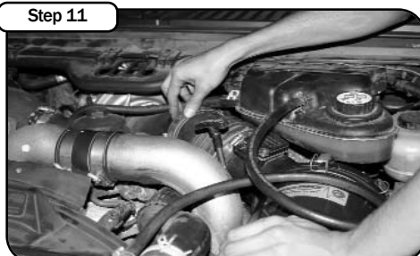
Step 11 Tighten the clamp on the turbo inlet. Reconnect the MAF sensor wiring harness and the filter minder harness.
