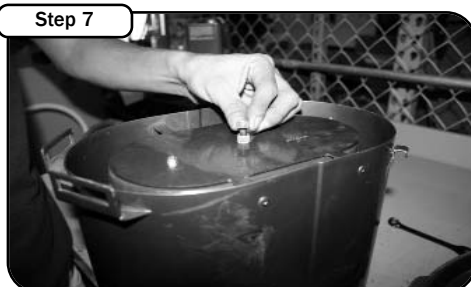
Step 7 Assemble the air filter housing by placing the new air filter inside the housing. Secure filter to housing with the provided nuts and washer. NOTE: The outer nut is used as a lock nut to secure filter.
