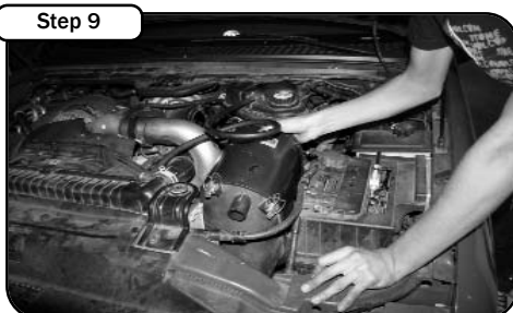
Step 9 Position the inlet side of the air box assembly into the engine bay.
