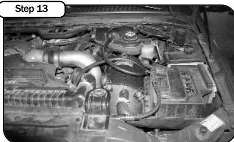
Step 13 Place enclosed CARB EO sticker on a clean/smooth surface on or near the intake system. EO identification label is required in passing Smog Check inspection. Your installation is now complete. Make sure you tighten all clamps and check all electrical connections. Re check periodically
