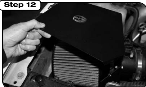
Step 12 Place cover on top of housing and fasten securely using 3 supplied 1/4-20x3/4 bolts and washers. For stage 1 kits, make sure all clamps are tight and all components are secure. Check and retighten connections and filter after a few hours of operation. (End of stage 1 installation instructions.)
