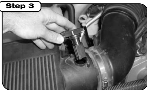
Step 3 Remove two screws that hold mass air flow sensor to stock airbox using supplied torx bit and remove sensor from airbox.
