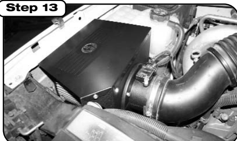
Step 13 Complete Stage 1 kit installed, for stage II kit instructions, continue on to step 14 and 15.
