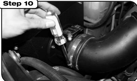
Step 10 Reconnect stock intake tube to Housing. Fasten securely. Also reconnect MAF sensor harness.
