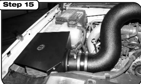
Step 15 Complete Stage 2 kit installed. Make sure all clamps are tight and all components are secure. Check and retighten connections and filter after a few hours of operation.
