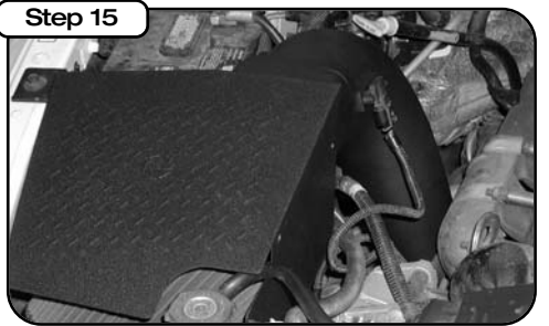
Complete intake kit installed. Be sure to re-check connections and re-tighten after a few hours of operation.
