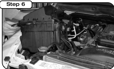
Remove factory airbox. Remove the 2 rubber mounting grommets.
