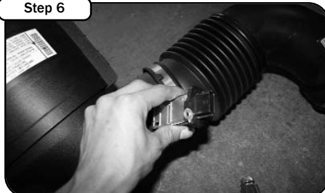
Step 6 Take out factory MAF sensor using the supplied torx T-20 bit to unscrew bolts. Be careful in handling the MAF sensor.
