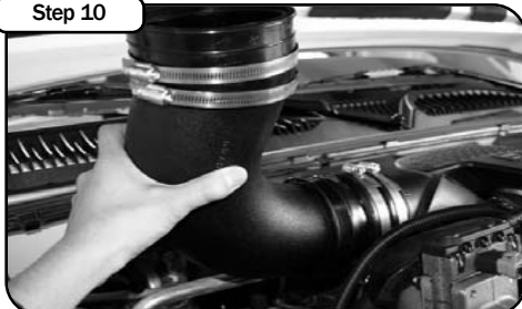
Step 10 Install 4 3/4" coupler onto 05-00749 tube, using clamps provided. Place 4 1/4" coupler on turbo side with clamps and install tube.
