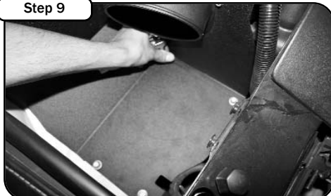
Step 9 Install new aFe housing. Use factory 10mm screws to secure the housing. Tighten all four screws.
