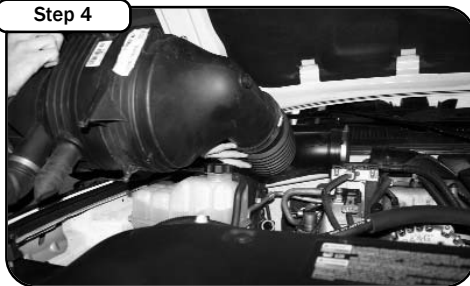
Step 4 Remove airbox. Grab from MAF area, (not directly on MAF) and pull up. It is held in place with rubber grommets.
