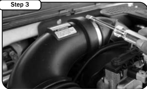
Step 3 Disconnect factory MAF sensor harness. Loosen the factory intake tube with a 5/16" nut driver.
