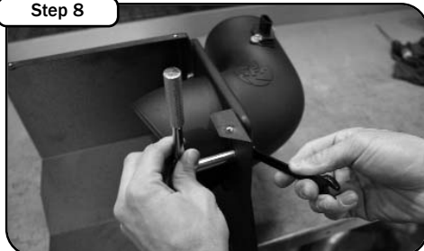
Step 8 Install 05-00890 tube outside of the housing using screws, washers, and nuts provided. Tighten all screws with 7/16" and 3/8" wrench or socket.
