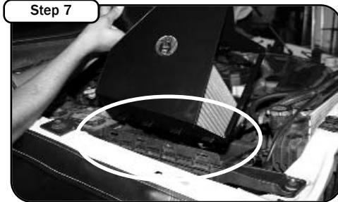
Step 7 Make sure the alignment hinges fall into the grooves on the lower OEM air box.
