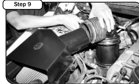
Step 9 Insert and secure the stock air intake tube onto the aFe housing.
