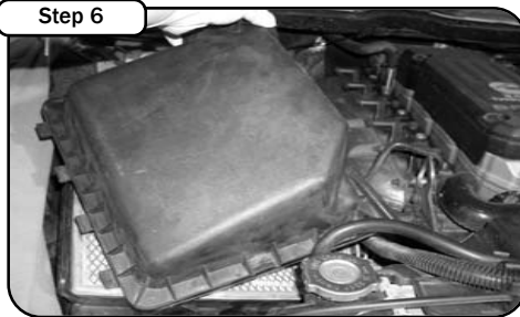
Step 6 Un-clip and remove the upper air box and stock air filter.
