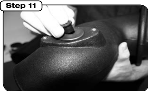
Step 11 If vehicle is equipped with an air temperature sensor, use grommet in the MAF sensor opening and insert air temperature sensor into grommet. The grommet is a tight fit and may be difficult to insert.
