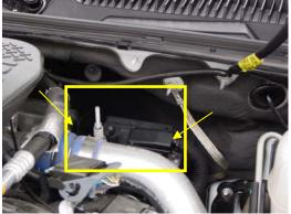
1. **View Glow Plug Controller** mounted on Driver Side Firewall. Remove 2 bolts holding the controller case cover.
