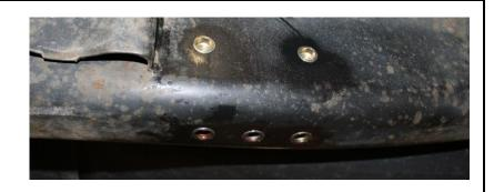
11. Mount both frame mount brackets to the frame using the 3/8"-16 serrated flange bolts.Use blue thread lock on all bolts and torque to 40 ft-lbs.
