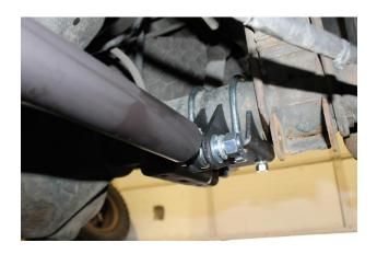
5. Ensure the vehicle is positioned on level ground with an empty bed to locate the at-rest frame mount location. Place the frame mount firmly against the frame. Start one pilot location hole using the 27/64" drill bit. Once the drill hole location has been clearly marked you may use a smaller drill bit to create the pilot hole.
