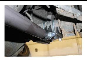
14. Torque the <sup>3</sup>⁄<sub>4</sub>"-16 jam nuts to 145 ft-lbs. Use a flat head screwdriver to centre the rod end during torqueing.
