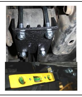
Install the traction bars into the axle mount using the ¾"-16 X 2.5" bolts. Do not torque at this time.
