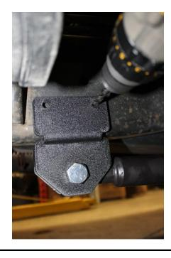
Gradually increase the drill bit size until the hole is 17/32" (0.531") in diameter. Deburr or smooth the leading edge of the drilled hole and apply a small amount of paint to resist corrosion.
