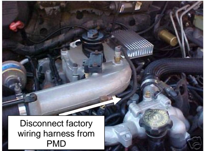
and then push it off. Pull up the wiring harness connector. For extended reach you can slice the outer loom to allow a little more wiring harness length.
