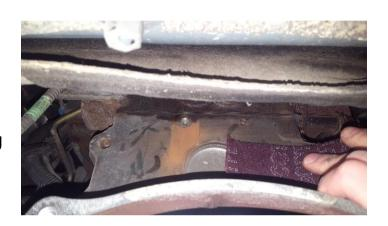
3. Make sure the M8 and M12 bolts can be threaded in by hand. You may need to run a thread chaser down the bolt holes or use penetrating fluid.
