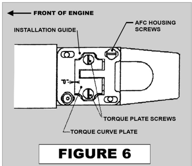
23) Install one of the two torque plate screws and hand tighten as tight as possible with a normal large screwdriver. Install the second screw. Using the hand impact tool and a large standard bit, tighten each screw another 1/8" to 1/4" turn.
