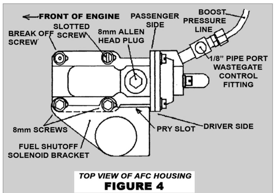
13) Use the hand impact tool and a 8mm socket to remove the two drivers side AFC screws.
