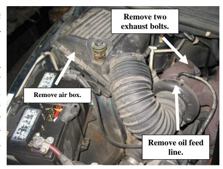
Remove the turbo oil feed line and un-bolt the turbo oil drain tube and cover the inlet to protect it from contamination.
